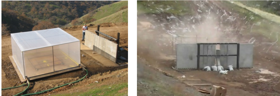
Fig.2 Experiment of hydrogen explosion and RC structure damage (left:Experimental system, right:A moment of explosion)
