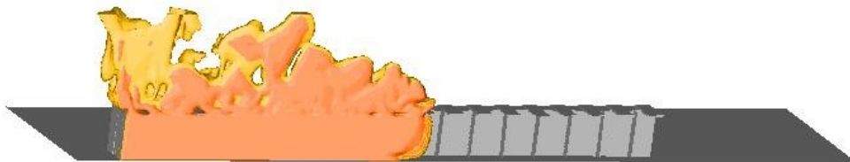
Figure 1-99 Computational Fluid Dynamics can be useful when estimating required venting. Distributed venting, like the transverse venting shown above [Hansen, 2005], can be very efficient to keep pressures low. CFD-tools can take into account detailed layout, including shape of vessel, position and shape of vent openings, presence of geometry and more. In addition to maximum pressure, shape and duration of pressure as well as distribution in space can be found using CFD.
